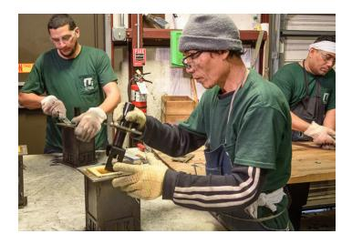
Locating a metal insert precisely into a urethane part can be challenging, but due to the production quantities needed, having the ability to place the insert in a matter of seconds was very important. At one point UI was creating 16,000 pieces of dunnage a week over two shifts. Anything UI or GM could do to improve process time was implemented.
