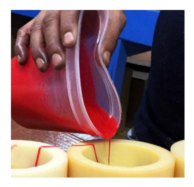
Once the mold concept was modified to accept the ring, the UI team had to figure out how to keep it in place during casting and curing.
